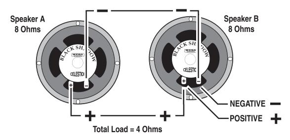
COMBINATION OF SERIES & PARALLEL: This is really just two sets of Series wired speakers connected in Parallel. This is how you maintain a consistent load with multiple speakers. The importance of this is more evident when you have more than one cabinet to connect to your amplifier. This is when you need to figure out the loads and how to wire them up without applying too low of a resistance on the amplifier.
